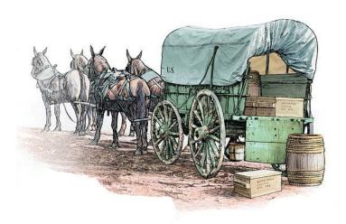
these wagons was based upon the sturdy farm wagons used in Pennsylvania. The dimensions of the box of these useful vehicles were as follows: Length (inside), 120 inches; width (inside) 43 inches; height, 22 inches. each wagon had its own
